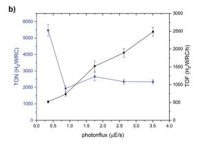
Fig. 5 TON and maximum TOF for H $_2$  evolution vs. (a) WRC concentration at a constant photon flux of 0.35  $\pm$  0.02  $\mu\text{E s}^{-1}$ . (b) photonflux with 10  $\mu\text{M}$  of WRC. Experimental conditions: 10 mL of solution, 0.500 mM [Ru(bpy) $_3$ ]Cl $_2$ , 0.1 M NaAscO, 0.1 M TCEP, pH 5.0, 453 nm LED irradiation. Black circles denote the maximum TOF of H $_2$  production and blue squares the turnover numbers.
