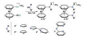
Scheme 3 Reaction scheme for conjugation of five and sixmembered N-heterocyclic rings to  $[Re(\eta^6-C_6H_6)(\eta^6-C_6H_5Cl)](PF_6)$  and  $[Re(\eta^6-C_6H_5Cl)_2](PF_6)$ . Reaction conditions: (1) Deprotonation of the N-heterocyclic rings or 2,2'-dipyridylamine with NaH, 2 h, 60 °C, THF; (2) nucleophilic substitution 3 h, 60 °C, THF.
