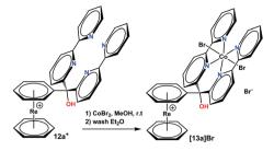
Scheme 6 Synthesis of complex [12a]Br. Reaction conditions: (1) 20 eq. CoBr2, 1 h, r. t., in MeOH, (2) several washes with Et2O.
