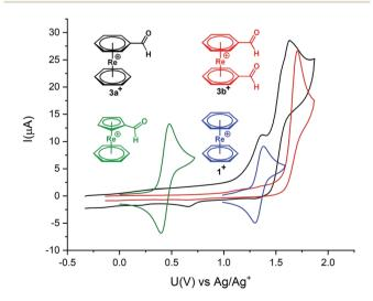
Fig. 1 Cyclovoltammogram of complexes  $1^+$  (blue),  $3a^+$  (black),  $3b^+$  (red) and mixed sandwich arene-Cp aldehyde (green); acetonitrile, 0.1 M [TBA][PF $_6$ ] (electrolyte), glassy carbon working electrode (i.d. = 3 mm), Pt auxiliary electrode, and Ag/AgCl reference electrode, analyte concentrations 1 mM, voltage step: 6 mV, sweep rate: 0.1 V s $^{-1}$ .
