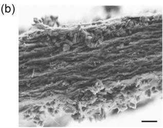
Fig. 3 SEM micrographs of (a) the surface and (b) the fracture crosssection of the 1:1:1 HNT-SEP-CNF hybrid nanopaper, respectively. The scale bars refer to  $2 \mu m$ .
