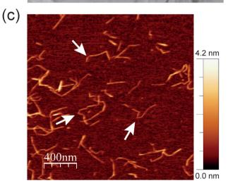
Fig. 2 SEM micrographs of (a) neat HNTs (white arrows represent the hexagonal kaolin sheets), (b) neat sepiolite and (c) the AFM image of the CNF (white arrows represent the fiber kinks). The scale bars in (a) and (b) refer to 500 nm.
