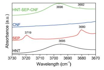
Fig. 5 FTIR spectra of the HNT, SEP, CNF and HNT-SEP-CNF hybrid nanopaper (3730-3670 cm<sup>-1</sup> range). The complete spectra are provided in Fig. S3.†
