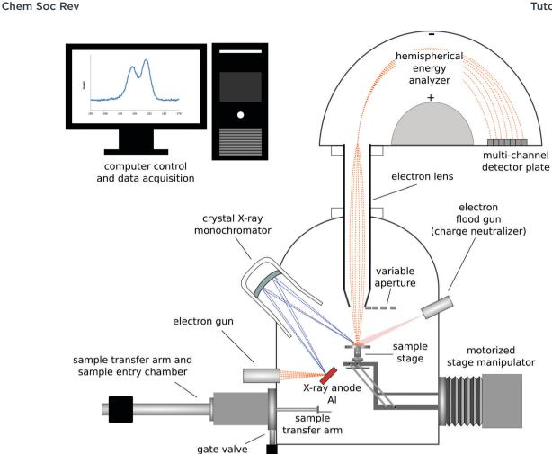
Fig. 1 Schematic drawing of a monochromatized XPS instrument with a hemispherical analyzer and multi-channel detector.
