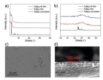
Fig. 3 (a) PXRD patterns of simulated TpBpy (black), TpBpy film (red), and TpBpy-Ni film (blue), (b) zoomed-in figure of 18-35° region in (a), (c) topview SEM image of TpBpy-Ni film, (d) cross-section view SEM image of TpBpy-Ni film.
