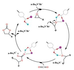
Scheme 2 Proposed mechanism of CO<sub>2</sub> cycloaddition via HMOF 2 and TBAB as a co-catalyst.
