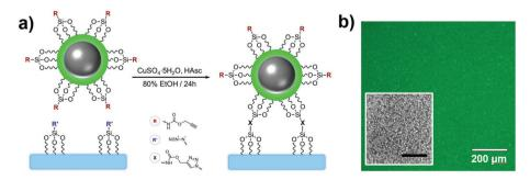
Fig. 10 (a) Grafting scheme of Ag@(FL) NPs to a SiO $_2$  substrate through Cu<sup>I</sup>-catalyzed 1,3-dipolar cycloaddition. (b) Fluorescence image of the substrate grafted with Ag@(FL) NPs ( $\lambda_{exc} = 489 \pm 6$  nm,  $\lambda_{em} = 536 \pm 20$  nm). Inset: SEM image of a region the substrate (scale bar: 1 µm). Adapted from ref. 115 with permission from the Royal Society of Chemistry, Copyright 2014.
