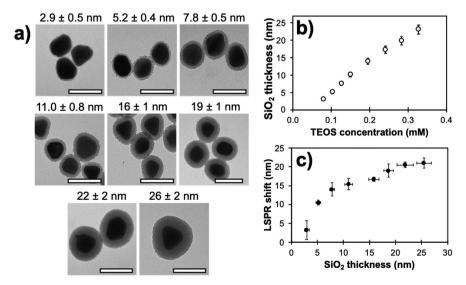
Fig. 3 (a) Transmission electron micrographs of (60 ± 8) nm Ag cores with different silica shell thicknesses (scale bar: 100 nm). (b) Experimental SiO<sub>2</sub> shell thickness on the (60 + 8) nm Ag cores presented in (a) in relation to TEOS concentration during synthesis. (c) Corresponding LSPR shift as a function of the shell thickness. Modified from ref. 94 with permission from Springer Nature, Copyright 2016.
