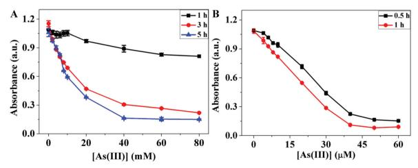
Fig. 5 The absorbance of the (A) GSH-DTNB, and (B) DTT-DTNB mixtures in the presence of different concentrations of As(III) at different reaction times.
