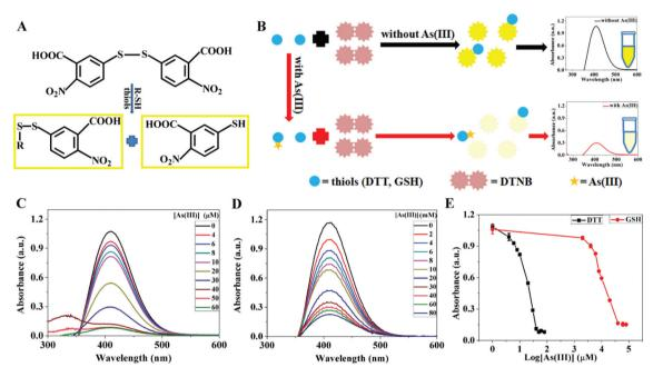
Fig. 4 (A) The reaction between free thiol and DTNB producing yellow products. (B) A scheme of reactions between thiols and DTNB without and with As(III). (C) The UV-vis spectra of DTT-DTNB mixture in the presence of different concentrations of As(III) (reaction time: 1 h). (D) The UV-vis spectra of GSH-DTNB mixture in the presence of different concentrations of As(III) (reaction time: 3 h). (E) The absorbance of the DTT-DTNB and GSH-DTNB mixtures at different concentrations of As(III).
