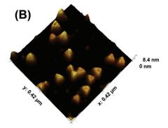
Fig. 1 Structural characterizations of Au TNPs. (A) A representative scanning electron microscopy image of Au TNPs attached onto a silanized glass substrate. Scale bar is 100 nm. (B) An atomic force micrograph of Au TNPs.
