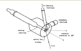
Fig. 10 Example of a stationary electrochemical cell used for Raman experiments. Reprinted from the original work by Fleischmann et al., 120 Copyright 1974, with permission from Elsevier.
