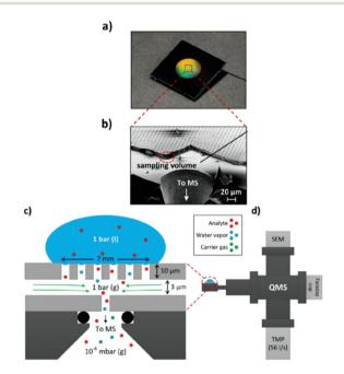
**Fig. 24** Membrane DEMS setup for thin-layer cell; (a) membrane chip photograph; (b) scanning electron microscope image of the membrane chip; (c) schematic of the membrane chip; (d) schematic of the setup. Image reprinted and modified with permission from Trimarco *et al.*<sup>301</sup> Copyright 2018 American Chemical Society.
