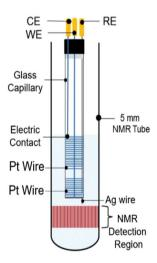
**Fig. 18** Schematic of a coil-based three-electrode NMR-SEC cell. Reprinted from the original work by da Silva *et al.*, <sup>275</sup> Copyright 2019, with permission from Elsevier.
