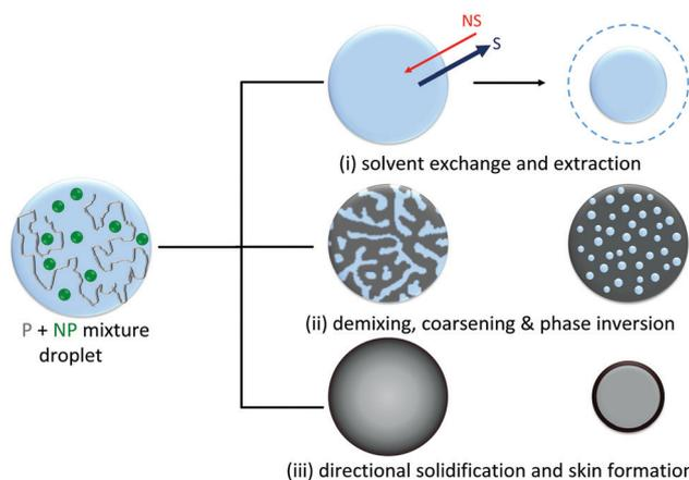
**Fig. 2** Schematic of the capsule formation mechanism, illustrating the three governing, simultaneous processes: (i) solvent exchange and extraction, resulting in drop shrinkage, (ii) droplet demixing, initiated by ingress of non-solvent, proceeding via spinodal decomposition or nucleation and growth, and (iii) eventual phase inversion and directional solidification, generally resulting in the formation of a smooth skin and internal microstructure.
