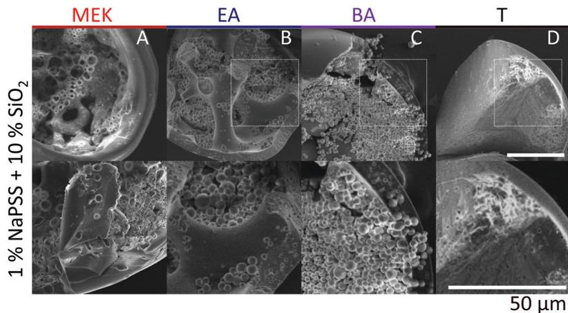
Fig. 7 SEM images of the internal microstructure of composite polymer–nanoparticle capsules obtained from droplets with initial concentration 1% w/v NaPSS + 10% w/v SiO<sub>2</sub> immersed in (A) methyl ethyl ketone, MEK, (B) ethyl acetate, EA, (C) butyl acetate, BA, and (D) toluene, T. Initial droplet radius  $R_0 \approx 250$ – $270 \mu\text{m}$  for all capsules. High magnification images of highlighted sections of the capsules are provided on the bottom row.
