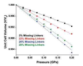
Fig. 7 Unit cell volume of UiO-66 as a function of pressure. Each sample exhibits different defect density. A more shallow slope indicates a higher bulk modulus, while steeper slopes correspond to lower bulk modulus values. Adapted with permission from ref. 62. Copyright 2019, American Chemical Society.
