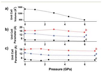
Fig. 6 (a) Unit cell volume of MIL-53(Al), (b) unit cell parameters of MIL-53(Al), and (c) unit cell parameters of NH<sub>2</sub>-MIL-53(Al) as a function of pressure. The parameter corresponding to the b-axis exhibits a notable increase at low pressures—an example of negative linear compression. Adapted from ref. 54 – published by the Royal Society of Chemistry.
