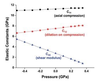
Fig. 2 Plot of ZIF-8 unit cell parameter and elastic constants vs. pressure.  $C_{11}$ ,  $C_{12}$ , and  $C_{44}$ , correspond to the moduli for axial compression, dilation upon compression, and shear, respectively. The precipitous decline in  $C_{44}$  indicates a drop in the shear modulus at elevated pressure, a phenomenon known as "shear-mode softening". Adapted with permission from ref. 24. Copyright 2013, American Chemical Society.
