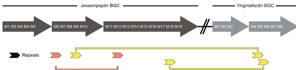
Fig. 8 Schematic representation of repetitive sequences in the jessenipeptin ( jes QS ) and virginiafactin ( vif ) BGC. red: jes QS -A6 Ala and jes QS -A12 Ala , yellow: jes QS -M9 Ser and vif QS -M5 Ser ; jes QS -M18 Ser and vif QS -M5 Ser (repetitive sequences were found using Repeat Finder of Geneious® Version 9.1.5).
