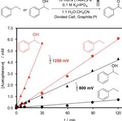
Fig. 4 Formation of acetophenone during the first two hours of (TAML)Fe catalyzed electrochemical oxidation of ethylbenzene (circles, 20 mM) or 1-phenylethanol (triangles, 20 mM) at applied potentials of 1250 mV (red) and 800 mV (black) (vs. Ag/AgCl) in 1:1 CH $_3$ CN: H $_2$ O and 0.1 M K $_2$ HPO $_4$  in a divided cell.
