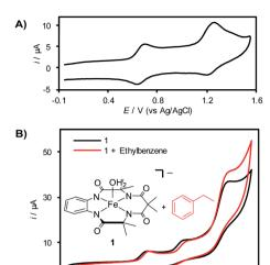
Fig. 1 (A) CV of  $[(TAML)Fe^{III}(OH_2)]Na$  (1) in  $CH_3CN$  (0.1 M LiClO<sub>4</sub>). (B) CVs of 0.5 mM 1 in the absence (black) and presence (red) of 20 mM ethylbenzene in 1:1 CH<sub>3</sub>CN: H<sub>2</sub>O and K<sub>2</sub>HPO<sub>4</sub> (0.1 M). The increase in the current of the (TAML)Fe redox feature at 1.25 V (vs. Ag/AgCl) is attributed to catalytic ethylbenzene oxidation by a high-valent Fe-oxo species generated at this potential. Scan rate = 50 mV s<sup>-1</sup>.
