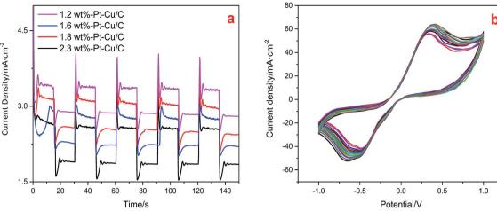
Fig. 10 Light and dark current densities of  $CO_2$  photoelectrochemical reduction system with four catalysts (1.2 wt% Pt-Cu/C catalyst, 1.6 wt% Pt-Cu/C catalyst, 1.8 wt% Pt-Cu/C catalyst, 2.3 wt% Pt-Cu/C catalyst) (a), stability test with 1.6 wt% Pt-Cu/C catalyst (b).
