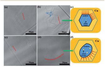
Fig. 3 Optical microscopy images of graphene domains after etching at 1000 °C for (a and b) 10 and (c) 15 min. The gas flow rate of etching was 2:50 (20 sccm  $\rm H_2$  and 500 sccm Ar). (d) Optical microscopy image of GED at 1050 °C. (e and f) Schematics of different etching results between GECRP and GED.
