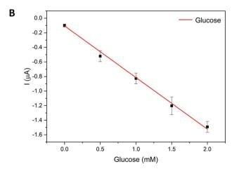
Fig. 5 Amperometric detection of glucose in the flow injection analysis system with 3D-PMED. (A) Amperometric current response at -0.1 V (vs. Ag/AgCl reference electrode) with alternant injecting of glucose (successive addition of 0.5 mM, 1.0 mM, 1.5 mM, 2.0 mM glucose) and PBS. (B) The calibration plot with the error bar ranging from 0 mM to 2.0 mM.
