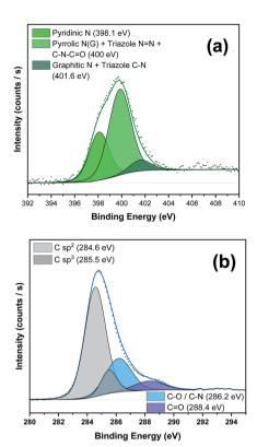
Fig. 3 (a) N 1s and (b) C 1s core level XPS regions of NG-PDI  ${\bf 1}$  and their relative fits.
