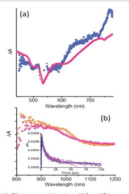
Fig. 6 (a) fs-TA spectra at a delay time of 1.5 ps of 5 (magenta) and 1 (blue). (b) fs-TA spectra of 5 (orange) at a delay time of 9 ps and 1 (magenta) at a delay time of 1.7 ps. All spectra were recorded in DMF at the excitation wavelength of 535 nm corresponding to the main absorption of PDI of the hybrid. The (b) inset shows the kinetic profile of the 965 nm peak corresponding to PDI\*. Note: the intensities are not drawn to scale.
