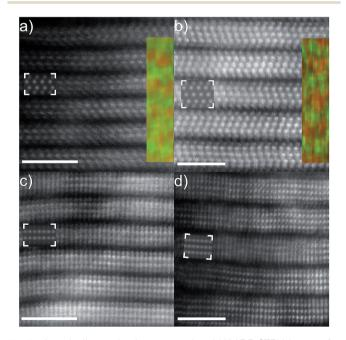
Fig. 2 Atomically resolved cross-sectional HAADF-STEM images for {11–20} oriented (a)  $T_{i_2}CCl_2$  and (b)  $T_{i_3}C_2Cl_2$ , and for {1–100} oriented (c)  $T_{i_2}CCl_2$  and (d)  $T_{i_3}C_2Cl_2$ . The colored insets in (a) and (b) correspond to lattice resolved EDX elemental maps showing  $T_i$  (red) and  $C_i$  (green). Note that the insets are showing simulated cross-sectional STEM images of  $T_{i_2}CCl_2$  and  $T_{i_3}C_2Cl_2$  for each orientation. Scale bars correspond to 2 nm.
