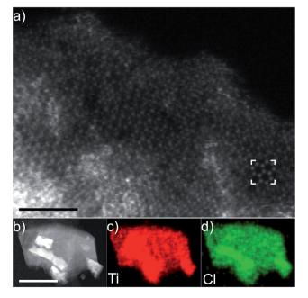
Fig. 1 (a) Atomically resolved plan-view HAADF-STEM image of a Ti<sub>2</sub>CT<sub>x</sub> MXene multilayer particle and (b) a low magnification overview with corresponding (c) Ti and (d) Cl elemental maps. Note that the inset in (a) is showing a simulated plan-view STEM image of Ti<sub>2</sub>CCl<sub>2</sub> (middle right). The scale bar in (a) corresponds to 2 nm and in (b) it corresponds to 0.5 µm.
