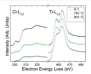
Fig. 4 Electron energy loss spectroscopy from a thin edge of a  $Ti_3C_2T_2$  multilayer particle, showing the background subtracted and multiple scattering deconvolved Cl- and  $Ti-L_{3,2}$  edges under ambient conditions and after heating at 750 and 800 °C. The spectra are normalized against the  $Ti-L_2$  peak maximum and vertically separated for clarity.
