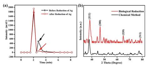
Fig. 3 (a) Chromatographic profiling of the Fagonia cretica extract before and after reduction and (b) XRD spectra of Ag NPs synthesized using the Fagonia cretica extract and chemical method.
