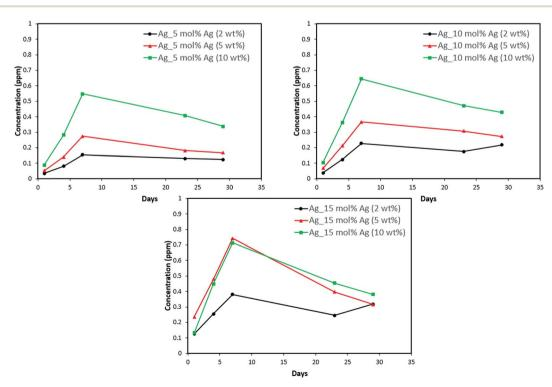
Fig. 12 Silver release from adhesive resin disc specimens containing 5, 10 and 15 mol% silver with different weight fractions of silver-ACP.
