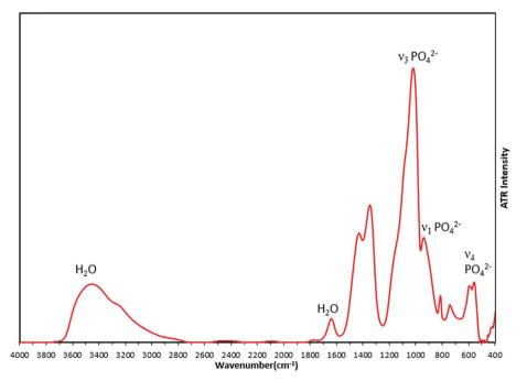
Fig. 8 FTIR spectrum of the synthesized particles (5 mol% silver).
