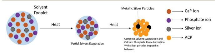
Fig. 2 Pictorial depiction of formation of silver-containing ACP nanoparticles. The solvent droplet initially contains all the ions in solution. As the droplet passes through the heated tube, solvent evaporates, after which calcium and phosphate ions react and precipitate to form the ACP phase, with silver nanoparticles becoming trapped within that phase.
