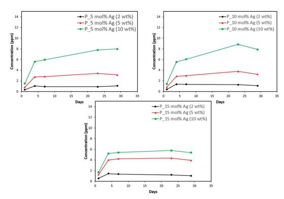
Fig. 11 Phosphorus release from adhesive resin disc specimens containing 5, 10 and 15 mol% silver with different weight fractions of silver-ACP.
