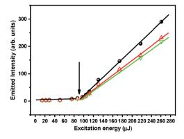
Fig. 5 RL emission intensity as a function of excitation energy for the samples studied: CA + 0% PEO (red up triangles), CA + 10% PEO (black circles) and CA + 20% PEO (down green triangles). The energy threshold is marked by the downward arrow, measured as 97 µJ. The experimental error in determining the excitation energies is  $\pm 10\%$ .
