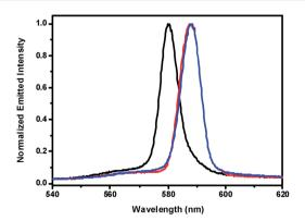
Fig. 6 Normalized random laser emission intensity of electrospun fibers as a function of incorporation of the additive PEO (0% – black line, 10% - red line and 20% - blue line) in the polymeric matrix of cellulose acetate. The pump energy was 5 mJ.
