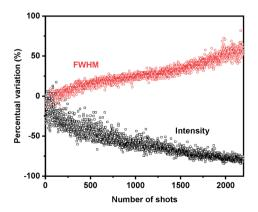
Fig. 9 Degradation behavior of the FWHM and intensity of RL as a function of the number of shots. The excitation energy was 5 mJ and the repetition rate was 1 Hz.
