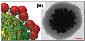
Fig. 3 Schematics of satellite adhesion onto (A) PAH coated and (B) branched PEI coated core particles. Representative TEM images of the corresponding nanoassemblies are also shown.
