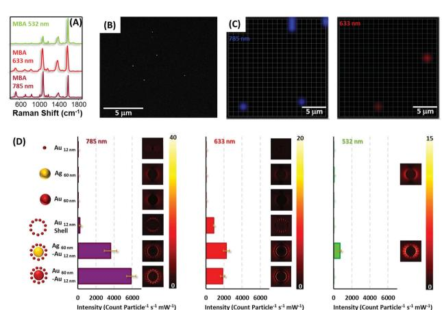
Fig. 5 (A) SERS spectra of MBA at different laser lines on  $Au_{core}@Au_{satellites}$ . (B) Example of a SEM image of a sample spin-coated with a diluted solution of  $Au_{core}@Au_{satellites}$ . (C) SERS imaging of the sample with 785 and 633 nm laser lines. Acquisition time 0.5 s. (D) SERS intensity, normalized for a single particle, provided by each material at three laser lines: 785, 633 and 532 nm. Simulation of the electric field maps provided by each of the materials.
