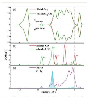
Fig. 4 DOS distribution of the Rh-MoSe $_2$ /CO system. The dashed line is the Fermi level. In the gas DOS, the red value shows the orbitals of isolated molecules while the green one shows the orbitals of adsorbed molecules.
