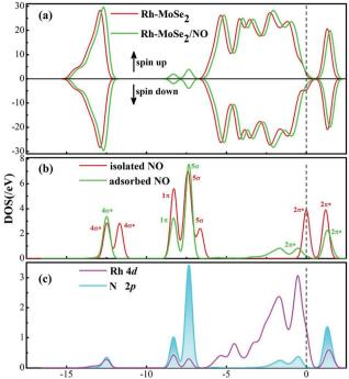
Fig. 6 DOS distribution of the Rh-MoSe<sub>2</sub>/NO system. The dashed line is the Fermi level. In the gas DOS, the red value shows the orbitals of isolated molecules while the green one shows the orbitals of adsorbed molecules
