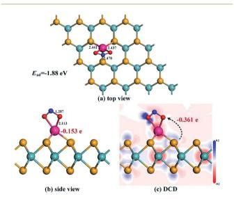
Fig. 7 Adsorption configuration (a) and (b) and DCD (c) of the Rh-MoSe<sub>2</sub>/NO<sub>2</sub> system.
