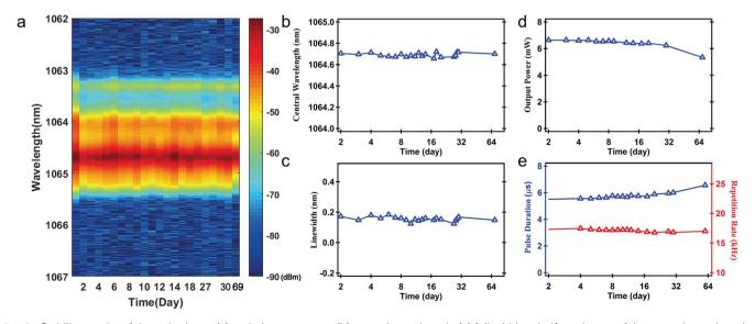
Fig. 6 Stability results of the pulse laser: (a) emission spectrum, (b) central wavelength, (c) full width at half maximum of the central wavelength, (d) output power, and (e) repetition rate and pulse duration at different time intervals.
