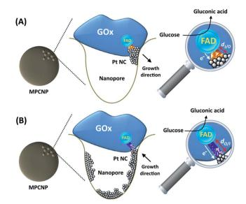
Scheme 1 Illustrations corresponding to the suggested configurations of (A) the inside-out enzymatically synthesized PtNC@GOx/MPCNP electrode and (B) the outside-in electrochemically synthesized PtNC-GOx/MPCNP electrode.
