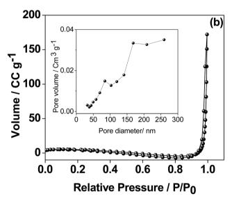
Fig. 10 Nitrogen adsorption and desorption isotherms and inset BJH adsorption pore size distribution of CaMoO $_4$  synthesized at (a) 300 and (b) 500 °C. The isotherms for the two are quite similar while the pore size distribution is quite different – note different pore diameter scaling in the insets.
