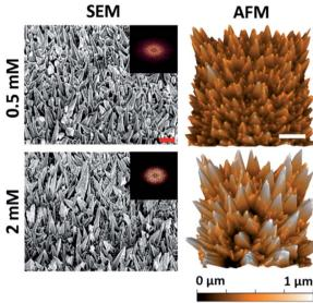
Fig. 3 Native surface data for the Pb $^+$  concentration series: column (1) SEM (45 $^\circ$  tilted) and column (2) AFM images of the gold nanospike surfaces for 0.5 and 2 mM Pb(CH $_3$ COO) $_2$ . The 2D-FFT data is shown for the top-down SEM images (see Fig. S5 $^+$ ). The red and white scale bars are 200 nm and 1  $\mu$ m, respectively.
