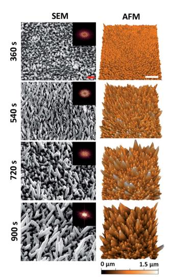
Fig. 1 Native surface data for the nanospike deposition series: column (1) SEM (45° tilted) and column (2) AFM images of the gold nanospike surfaces as a function of electrodeposition time. The red and white scale bars are 200 nm and 1  $\mu$ m, respectively. 2D-FFT data (insets) are shown for the top-down SEM images (see Fig. S2†).
