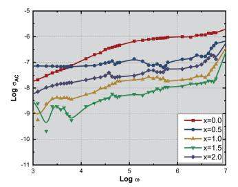
Fig. 9 Variation of AC conductivity with frequency of all the Ce<sup>3+</sup>-substituted YIG samples.
