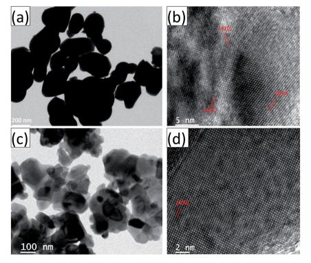
Fig. 5 (a) and (b) are the HRTEM and high-magnification images, respectively, of polycrystalline YIG, x = 0.0; (c) and (d) are the HRTEM and high-magnification images, respectively, of preferred  $\langle 100 \rangle$  oriented single-crystalline Ce-YIG, x = 2.0.
