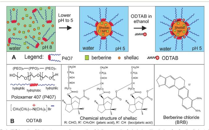
Fig. 1 (A) Schematics of the two step process for preparation of shellac nanocarriers for berberine with cationic surface functionality by steric stabilisation with Poloxamer 407 (P407) and doping with the cationic surfactant octadecyltrimethylammonium bromide (ODTAB). (B) Molecular structures of the constituting materials for preparation of antimicrobial shellac nanocarriers for berberine (BRB): Poloxamer 407 (P407), octadecyltrimethylammonium bromide (ODTAB), shellac and berberine chloride.
