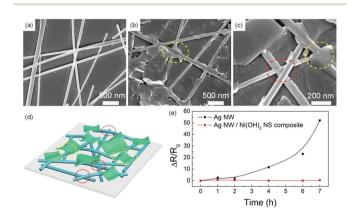
Fig. 4 SEM images of Ag NW (a) and Ag NW/Ni(OH)<sub>2</sub> NS (b and c) TEs. Schematic (d) of the Ni(OH)<sub>2</sub> NSs covering the NW junctions (yellow dashed circles) and the compressed connections of NW junctions (red dashed circles). (e) Variation of  $R_s$  of Ag NW and Ag NW/Ni(OH)<sub>2</sub> NS electrodes annealed at 200 °C as a function of annealing time.  $\Delta R = R$  $-R_0$ , where R and  $R_0$  are the  $R_s$  value after annealing, and the original  $R_s$  value, respectively.
