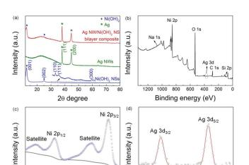
Fig. 2 XRD patterns (a) of Ni(OH)<sub>2</sub> NSs, Ag NWs, and the Ag NW/ Ni(OH)<sub>2</sub> NS composite. XPS of the Ag NW/Ni(OH)<sub>2</sub> NS composite: survey scan (b), Ni 2p (c) and Ag 3d (d) spectra.
