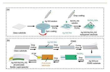
Scheme 1 Schematic of the fabrication of (a) the Ag NW/Ni(OH)<sub>2</sub> NS TE and (b) the all-solid-state flexible supercapacitor.
