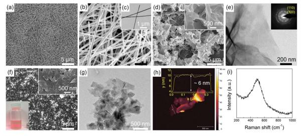
Fig. 1 SEM and TEM images of Ag NWs (a-c). SEM and TEM images of Ni(OH)<sub>2</sub> NSs before (d and e) and after (f and g) exfoliation. The inset in the lower-left corner of (f) is the photo of the exfoliated Ni(OH)<sub>2</sub> NS suspension. AFM image (h) with the corresponding height profile, and the Raman spectrum (i) of exfoliated Ni(OH)<sub>2</sub> NSs.
