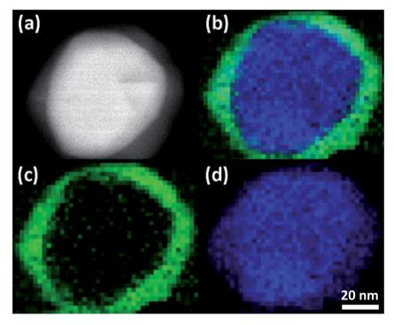
Fig. 1 The contrast of the HAADF image of a  $Ag_2S/Ag$  particles after 1 h (a) is sensitive to the atomic number difference between the  $Ag_2S$  and Ag domains. (b) Colorized EELS spectrum images from the same particle where green is sulfur (c) and silver is blue (d).
