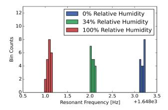
Fig. 5 Resonant frequency of a cantilever is shown for relative humidity values of 0, 34, and 100 percent (cantilever dimensions are: 3 mm long, 100 μm wide, 64 μm high, and a carbon infiltration time of 6 minutes). This histogram shows observations taken while humidity values were sequentially changed in a randomized order. Shifts on the order of 1 Hz were seen on top of a base resonant frequency of 1.65 kHz.
