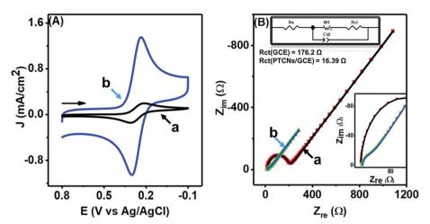
Fig. 6 (A) CVs and (B) EIS spectra of 5.0 mM  $K_3[Fe(CN)_6]$  in 1.0 M KCl at the GCE (a) and at the PTPCNs/GCE (b). The upper left side of (B) shows the Randel circuit, whereas the lower left inset shows the magnified EIS of the PTPCNs/GCE.
