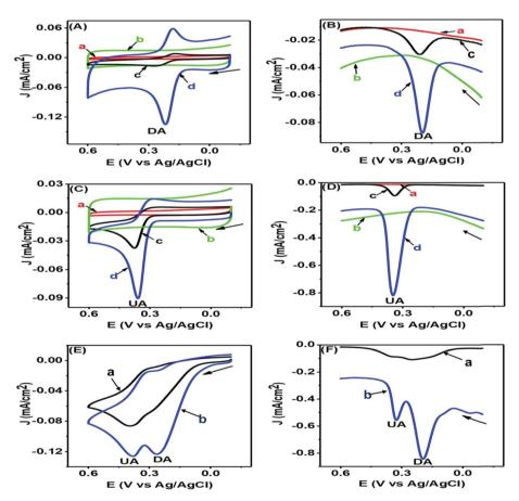
Fig. 7 CVs (A) and DPVs (B) of blank 0.1 M PBS solution of pH 7.0 (a and b) and 50  $\mu$ M DA (c and d) in the same PBS of pH 7.0 at the GCE (a and c) and PTPCNs/GCE (b and d). CVs (C) and DPVs (D) of blank 0.1 M PBS of pH 7 (a and b) and 200  $\mu$ M UA (c and d) in PBS of pH 7.0 at the GCE (a and c) and PTPCNs/GCE (b and d). CVs (E) and DPVs (F) of the mixture of 50  $\mu$ M DA and 200  $\mu$ M UA in 0.1 M PBS of pH 7.0 at the bare GCE (a) and PTPCNs/GCE (b).
