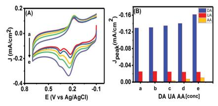
Fig. 10 (A) CVs and (B) peak current densities are shown for five different solutions containing fixed concentration of DA (50  $\mu$ M) and UA (100  $\mu$ M) with varying concentrations of AA (a–e): 100  $\mu$ M, 300  $\mu$ M, 500  $\mu$ M, 1 mM and 1.5 mM.
