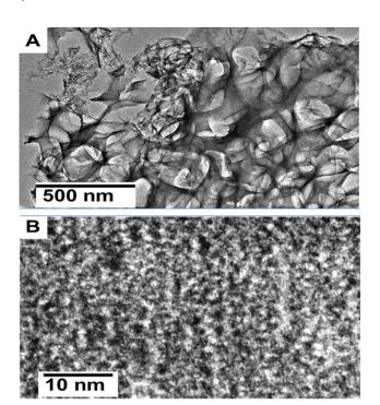
Fig. 2 (A) TEM and (B) HRTEM images of carbon nanosheets prepared from tal palm leaves at 850 °C.
