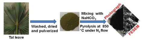
Scheme 1 Schematic representation for the preparation of PTPCNs from tal leaves at 850 °C.
