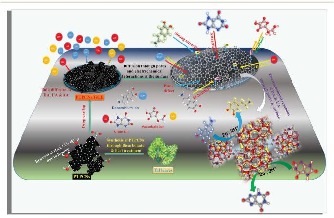
Scheme 3 Simple portrayal of the formation of pores in the PTPCNs, bulk diffusion of DA+, UA- and AA- at the PTPCNs/GCE, their interactions with the PTPCNs/GCE and electrochemical reactions of DA and UA through the surficial pores as well as the surface.
