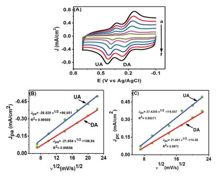
Fig. 8 (A) CVs of 50 μM DA and 200 μM UA at the PTPCNs/GCE in 0.1 M PBS of pH 7.0 at different scan rates (a-f): 50, 100, 200, 300, 400, 500 mV s<sup>-1</sup>. The relationship between the oxidation peak current densities (B) and reduction peak current densities (C) of DA and UA with the square root of the scan rates.
