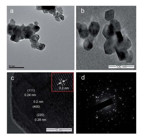
Fig. 3 TEM images of Co<sub>3</sub>O<sub>4</sub>/NiO-600 °C microspheres: (a and b) at high and low magnifications; (c) lattice plane; (d) SAED pattern.
