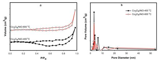
Fig. 6 Co<sub>3</sub>O<sub>4</sub>/NiO microspheres: (a) N<sub>2</sub> sorption isotherms; (b) micro- and mesopores distributions.
