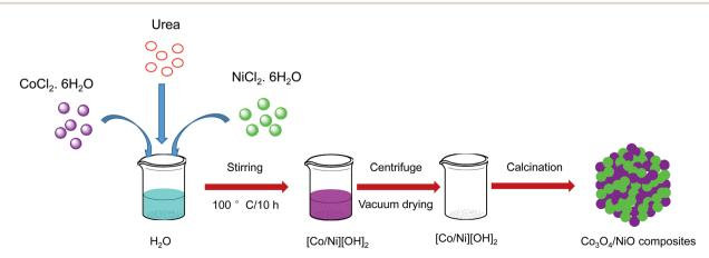
Fig. 1 Synthesis of flower-like 3D hierarchical Co<sub>3</sub>O<sub>4</sub>/NiO microspheres.
