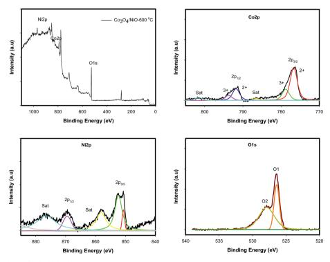
Fig. 5 XPS spectra of Co<sub>3</sub>O<sub>4</sub>/NiO-600 °C microspheres.
