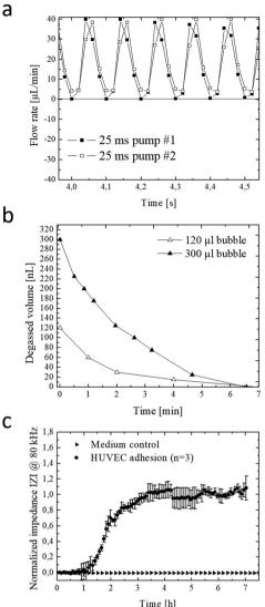
Fig. 2 (a) Peak flow profile of two parallel on-chip integrated micropumps for 25 ms actuation step time. (b) Removal of 120 nL and 30 nL air bubbles using the semi-permeable  $\mu degasser$  at -60 kPa negative pressure. (c) Representative impedance time-trace for endothelial cell adhesion and establishment of confluent endothelial monolayers during the first 7 hours of on-chip cultivation at a frequency of 80 kHz.
