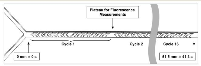
Fig. 2 Diagram of a micromixer channel, containing herringbone-shaped grooves in its surface. Two inlet channels are visible at the left. The channel is just over 50 mm long, and contains 16 cycles of 12 grooves each. Between cycles, a plateau is incorporated to allow for a 300 × 100 µm measurement region. At a total flow rate of 2.0 μL min<sup>-1</sup>, as used in the enzyme kinetics experiments, 51.5 mm channel length corresponds to a residence time of 41.3 s.
