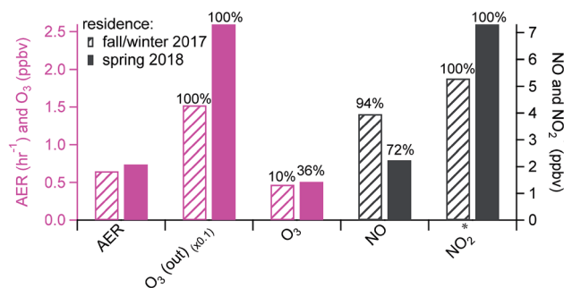
Fig. 2 Average AER, ambient outdoor O_3 levels, and mixing ratios of O_3 and nitrogen oxides in the residence under background conditions in two seasons. Data below the detection limit were included to calculate averages. Text above the bars indicates the percentage of data above the detection limit.
