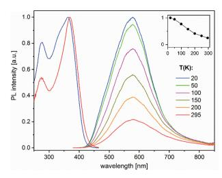
**Fig. 6** Photoluminescence excitation (PLE, left) and emission (PL, right) spectra of compound **8** in a temperature range between 20 and 295 K. The PLE and PL spectra were recorded and excited at 580 and 350 nm, respectively. The insert shows a temperature dependence of the integrated PL intensity.
