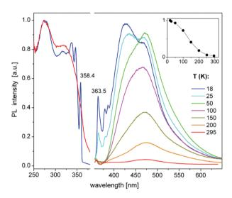
**Fig. 7** Photoluminescence excitation (PLE, left) and emission (PL, right) spectra of compound **9** in a temperature range between **18** and **295** K. The spectra were recorded and excited at **430** and **345** nm, respectively. The insert shows a temperature dependence of the integrated PL intensity.
