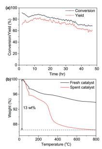
Fig. 6 (a) Stability test for Ni/Al $_2$ O $_3$ -PD catalyst.1-Hexanol at 1  $\mu$ L min $^{-1}$  with 8 mL min $^{-1}$  NH $_3$  and 20 mL min $^{-1}$  N $_2$  flowed through 200 mg catalyst at 230 °C. GHSV = 1.12 × 10 $^4$  h $^{-1}$ . (b) TG analysis for Ni/Al $_2$ O $_3$ -DP catalyst before and after reaction.
