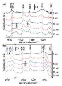
Fig. 4 DRIFTS of adsorbed species on NH<sub>3</sub> saturated Ni/Al<sub>2</sub>O<sub>3</sub>-DP surface as a function of time under  $N_2$  flow at 130 °C. At t = 0 min, (a) 1-butanol and (b) 1,1-dideuteriobutan-1-ol was injected.
