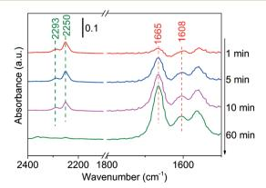
Fig. 5 DRIFTS of adsorbed butanenitrile on Ni/Al<sub>2</sub>O<sub>3</sub>-DP surface as a function of time under  $N_2$  flow at 100 °C. At t = 0 min, butanenitrile
