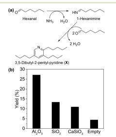
Fig. 1 (a) Scheme for formation of 3,5-dibutyl-2-pentyl-pyridine (compound X) and (b) yield of compound X with different supports. Reaction conditions: 1  $\mu$ L min<sup>-1</sup> hexanal, 200 mg catalyst, 190 °C, 8 mL min<sup>-1</sup> NH<sub>3</sub>, 20 mL min<sup>-1</sup> N<sub>2</sub>. GHSV = 1.12 × 10<sup>4</sup> h<sup>-1</sup>.
