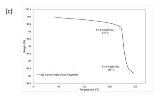
**Fig. 5** DSC and TGA traces of BES-0.5H2O. (a) DSC curve of a crystalline powder (black) and a single crystal (red). (b) TGA curve of a crystalline powder (black) including derivative with respect to time (red). (c) TGA curve of a single crystal form.
