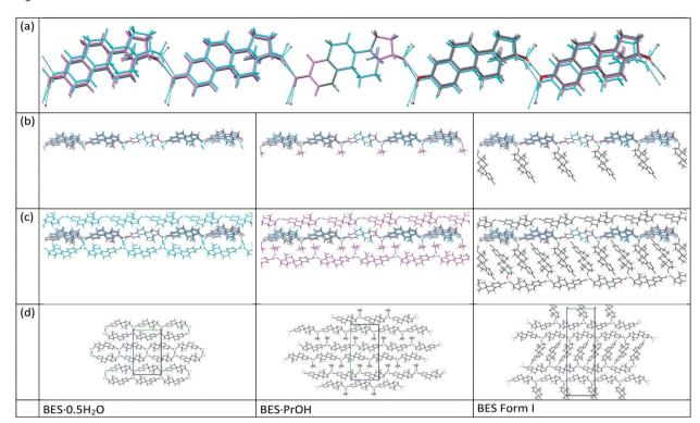
Fig. 9 Comparison of the common packings of BES Form I (coloured by element), BES-0.5H<sub>2</sub>O (cyan) and BES-PrOH (violet). (a) Shows the overlaid chain, (b) shows the chain and hydrogen bonded solvent (second BES molecule in the case of BES Form I), (c) shows the surrounding chains and (d) shows the crystal packing of each form.
