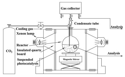
Fig. 1 Schematic of the experimental setup for the photoreduction of CO<sub>2</sub> with H<sub>2</sub>O
