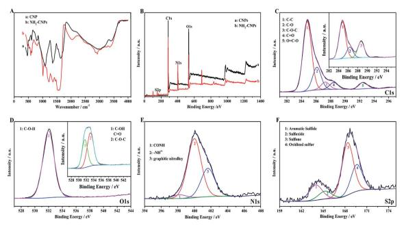
Fig. 4 Structural characterizations of CNPs and NH<sub>2</sub>-CNPs: (A) FT-IR spectra; (B-F) XPS spectra.
