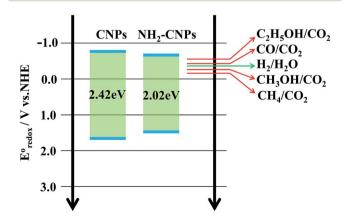
Fig. 8 Schematic of the mechanism of the photocatalytic CO<sub>2</sub> reduction with water on NH2-CNPs.
