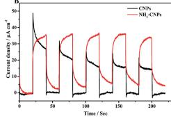
Fig. 7 (A) Nyquist plots of the CNPs (a) and NH<sub>2</sub>-CNPs (b). (B) The transient photocurrent responses of the CNPs (a) and NH<sub>2</sub>-CNPs (b) in 0.5 M  $Na_2SO_4$  aqueous solution under visible-light ( $\lambda > 420$  nm) irradiation.
