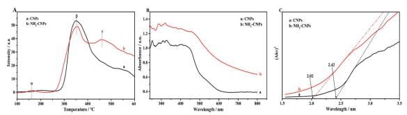
Fig. 6 (A) The CO<sub>2</sub>-TPD profiles of the CNPs (a) and NH<sub>2</sub>-CNPs (b), (B) DR UV-vis spectra of the CNPs (a) and NH<sub>2</sub>-CNPs (b). (C) The calculation of the band gap of the CNPs (a) and NH<sub>2</sub>-CNPs (b) based on the  $(Ahv)^2$  versus hv curve.
