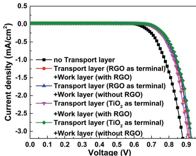
Fig. 7 Dark currents of devices with various photoanodes.
