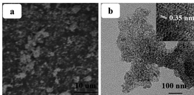
Fig. 9 SEM (a) and TEM (b) images of the RGO–TiO<sub>2</sub> scattering layer, the high magnification image of the material is shown in the inset.
