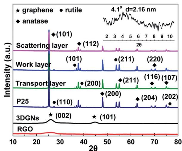
Fig. 2 XRD curves of the RGO, 3DGNs, TiO<sub>2</sub>, transport layer, work layer and scattering layer. The small angle XRD result of the transport layer is displayed as the inset.
