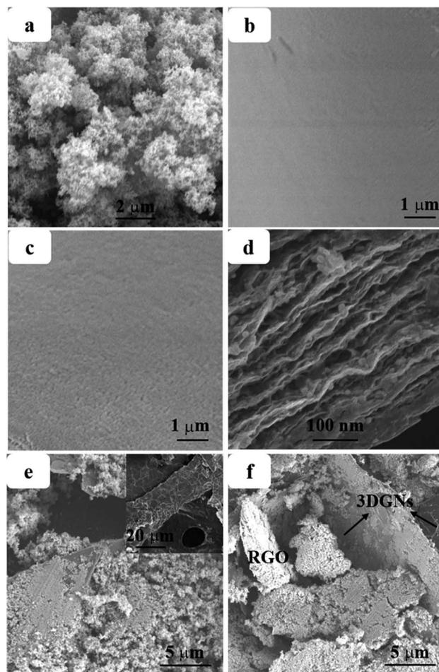
Fig. 1 SEM images of (a) TiO<sub>2</sub> (b) transport layer with the RGO as the terminal layer (c) transport layer with the TiO<sub>2</sub> as the terminal layer (d) cross-section view of the transport layer (e) the 3DGNs added work layer (the original 3DGNs shown in the inset) (f) the 3DGNs and RGO co-modified work layer.
