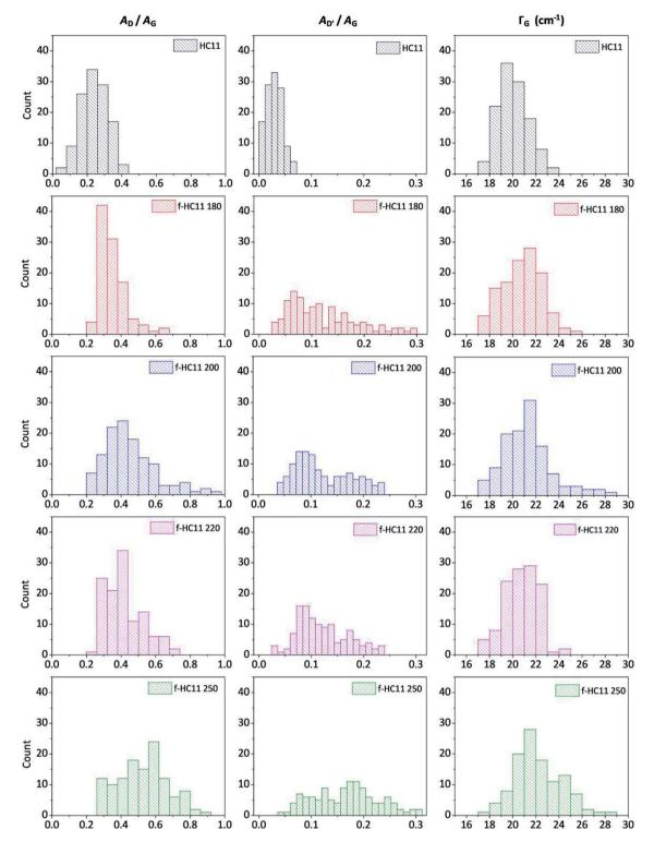
Fig. 4 Statistical analysis of the Raman spectra acquired from the HC11 and f-HC11 samples in terms of  $A_D/A_G$ ,  $A_{D'}/A_G$  and  $\Gamma_G$ .
