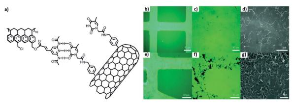
Fig. 22 (a) Chemical structure of PS1, thymine-MWCNTs; images of patterned surface by (b and e) fluorescence, (c and f) optical and (d and g) scanning electron microscopy, after deposition of a dispersion of Thymine-MWCNTs in DMF (b−d) and CHCl<sub>3</sub> (e−g).(Reproduced with permission from ref. 115 © 2012 American Chemical Society).
