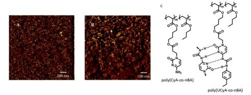
Fig. 13 AFM phase images for (A) poly(CyA-co-nBA); (B) poly(UCyA-co-nBA) films; (C) hydrogen bonding interactions in polymers. (Reproduced from ref. 92 with permission from The Royal Society of Chemistry).
