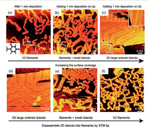
Fig. 4 STM images of: (a) 1D thymine filaments on Au(111) surface at low surface coverage, inset: structure of thymine; (b) 1D filaments and small islands; (c) extended 2D islands. Inset: magnified STM image of 2D island structure. (d–f) Images of STM tip manipulation experiment. (Reproduced with permission from ref. 72 © 2007 WILEY-VCH Verlag GmbH & Co. KGaA, Weinheim).
