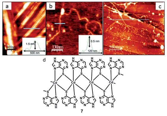
Fig. 28 (a) AFM image of crystals acquired by treating 7 with NaOH; (b) AFM image of a single polyanion; (c) AFM micrograph of fibers acquired by *in situ* reaction on HOPG; (d) structure of 7. (Reproduced with permission from ref. 127 © 2006, American Chemical Society).
