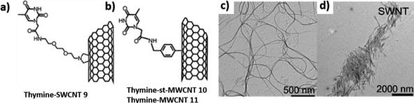
Fig. 21 Chemical structures of thymine-functionalised CNTs formed by: (a) 1,3-dipolar cycloaddition (b) arylation reaction. TEM images (c) 9 in DMF (d) 9 in DCM. (Reproduced with permission from ref. 114 The Royal Society of Chemistry).
