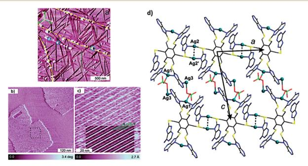
Fig. 25 (a) AFM phase image of ultrathin film of hexapodal silver complex 3 on HOPG surface. Graphite multiatomic terrace edges are shown in yellow dashed lines and with growth direction of rotational and mirror domains of 1D chains; (b) AFM constant height phase image of 2D domains; (c) high-resolution AFM topography image of black square region in (b); (d) plane containing Ag-coordinated polymer. (Reproduced with permission from ref. 120 © 2017 American Chemical Society).
