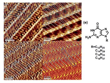
Fig. 5 Hydrogen bonded ribbons obtained from (a)  $C_{12}$ , (b)  $C_{14}$ , (c)  $C_{16}$ , and (d)  $C_{18}$  alkyl analogs of guanine by STM imaging; (e) structure of alkyl analogs of guanine. (Reproduced from ref. 77 with permission from The Royal Society of Chemistry).
