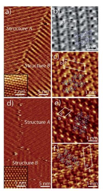
Fig. 15 Co-adsorption of adenine with L-serine (a–c) and with L-tyrosine (d–f) revealing pure adenine domains by STM imaging. (Reproduced from ref. 95 with permission from The Royal Society of Chemistry).
