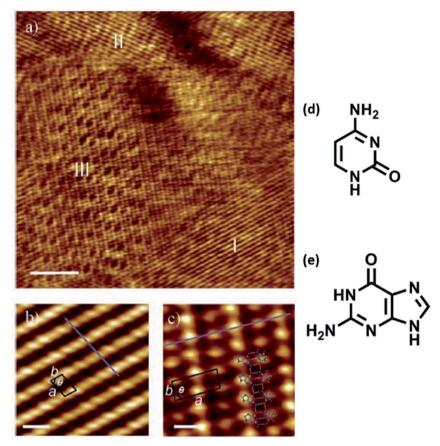
Fig. 7 Co-adsorption of cytosine and guanine on HOPG. (a) STM image displaying three distinct domains (labeled I–III), scale bar: 10 nm; (b) zoomed-in view of domain I structure, scale bar: 1 nm; (c) magnified view of domain III revealing an ordered array of high and low protrusions, scale bar: 1 nm; (d) structure of cytosine; (e) structure of guanine. (Reproduced with permission from ref. 83 ©2006, American Chemical Society).
