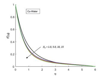
Fig. 9 Velocity distribution for various value of Nr when M=0.5, Pr = 0.3, Gr = 0.5, Ec = 0.1 and  $\lambda=1$ .
