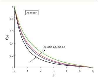
Fig. 2 Velocity distribution for various value of Ec when M=0.5, Pr=0.3, Gr=5, Pr=0.2 and Pa=0.2 a
