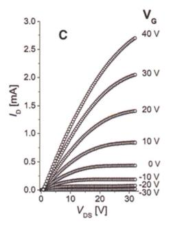
Fig. 4 The plot of drain current  $I_{\rm D}$  versus drain-source voltage  $V_{\rm DS}$  as a function of the gate voltage  $V_{\rm G}$  for an FET nanocrystal with a channel composed of 8 nm PbSe nanocrystals treated with hydrazine solution for 12 hours. Adapted with permission from ref. 47.
