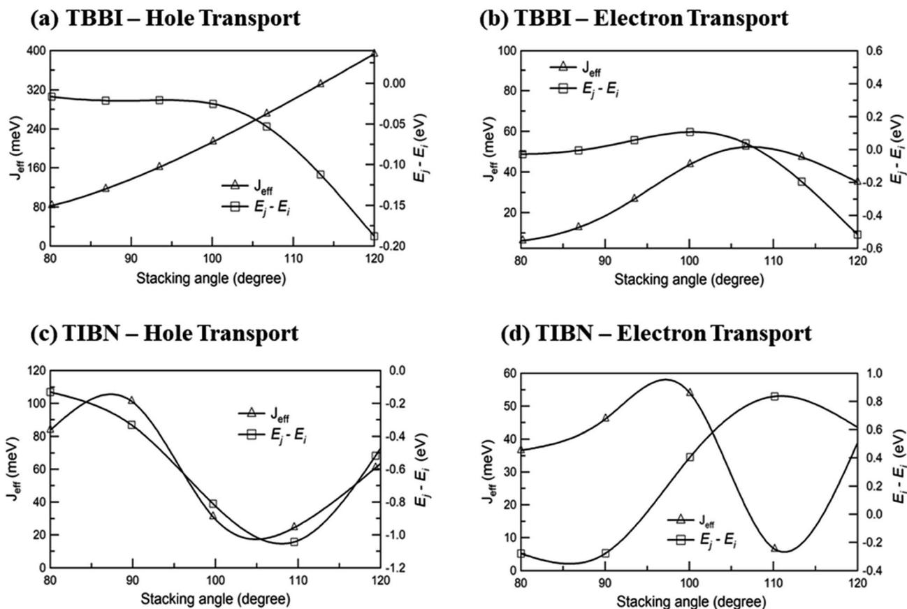
Fig. 3 Effective charge transfer integral ( $J_{\text{eff}}$ ) and energy difference between  $i^{\text{th}}$  and  $j^{\text{th}}$  sites ( $E_j - E_i$ ) for hole and electron transport of TBBI and TIBN molecules.
