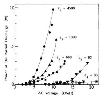
Fig. 7 Power of the partial discharge in the packed bed with different specific dielectric constant  $\varepsilon_{s}$ . Reproduced from ref. 219 with permission from Elsevier, copyright 1990.
