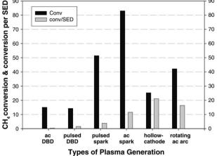
Fig. 1 Comparison of  $CH_4$  conversion rate and associated energy efficiencies for various plasma reactor types. Reproduced from ref. 77 with permission from Springer Nature, copyright 2013.
