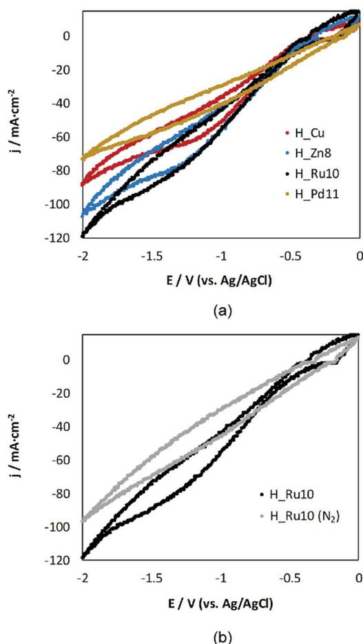
Fig. 5 Cyclic-voltammety responses for (a) H\_Zn8, H\_Ru10 and H\_Pd11 in comparison to H\_Cu-based GDEs in a medium saturated with CO<sub>2</sub> and, (b) responses for H\_Ru10 in the presence and absence of CO<sub>2</sub>.
