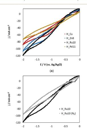
Fig. 5 Cyclic-voltammetry responses for (a)  $H_Z$ n8,  $H_R$ u10 and  $H_Z$ Pd11 in comparison to  $H_Z$ Cu-based GDEs in a medium saturated with  $CO_2$  and, (b) responses for  $H_R$ u10 in the presence and absence of  $CO_2$ .
