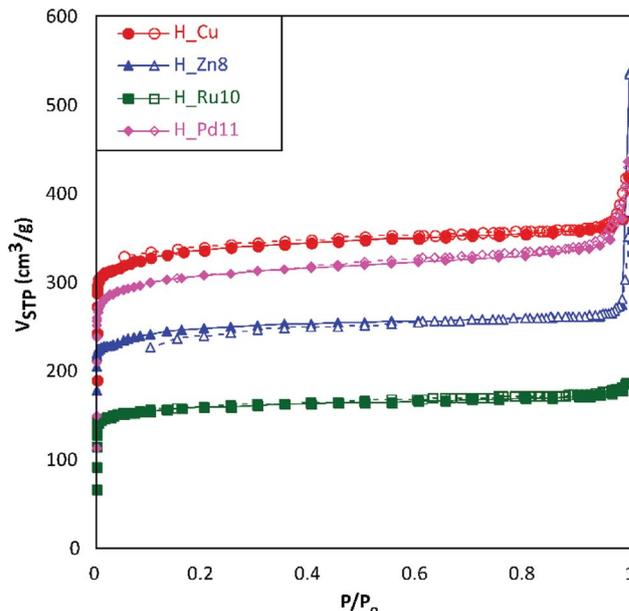
Fig. 4 N<sub>2</sub> adsorption isotherms at 77 K for H\_Cu, H\_Zn8, H\_Ru10 and H\_Pd11. Filled and empty symbols correspond to adsorption and desorption branches, respectively.
