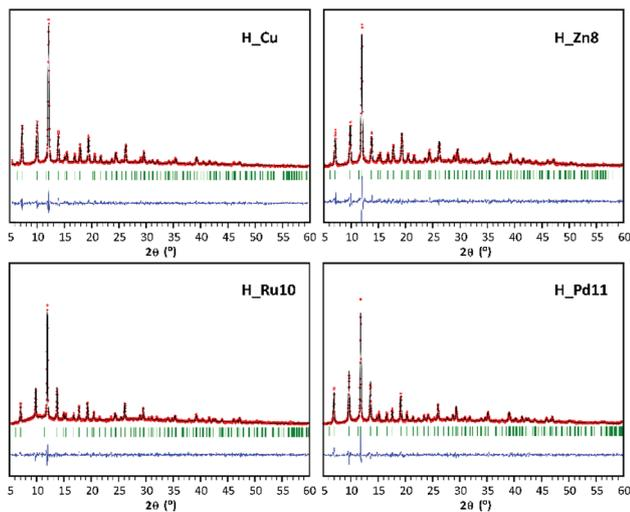
Fig. 1 PXRD pattern-matching refinement plots for H\_Cu, H\_Zn8, H\_Ru10, and H\_Pd11 (green ticks: calculated reflections; red circles: experimental pattern; black line: simulated pattern; blue line: difference between patterns).
