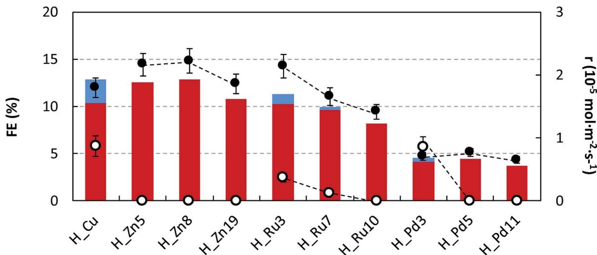
Fig. 7 FEs for  $\text{C}_2\text{H}_5\text{OH}$  (in red) and  $\text{CH}_3\text{OH}$  (in blue) formation and  $r$  for  $\text{C}_2\text{H}_5\text{OH}$  (●) and  $\text{CH}_3\text{OH}$  (○) in the electrocatalytic reduction of  $\text{CO}_2$  at H\_Zn, H\_Ru and H\_Pd in comparison to H\_Cu.
