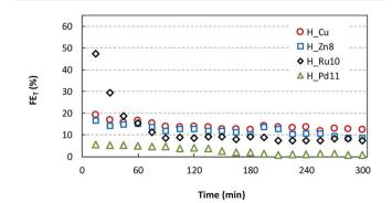
Fig. 6 Time-dependence of FE for H\_Zn8, H\_Ru10 and H\_Pd11 materials, in comparison to H\_Cu.
