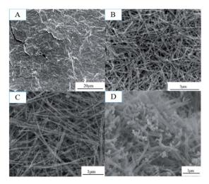
Fig. 1 SEM images of (A) GO, (B) GO/MnO<sub>2</sub>, (C) GO/MnO<sub>2</sub>/Fe<sub>3</sub>O<sub>4</sub>, and (D) GMFP nanocomposites
