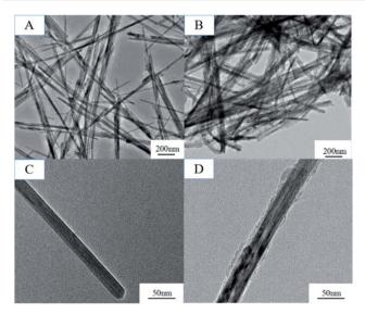
Fig. 2 TEM images of (A) and (C) MnO<sub>2</sub>, (B) and (D) MnO<sub>2</sub>/PPy.
